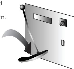
5. Press pedal forward to increase speed or backward to decrease speed. Press fully back to stop the wheel.
