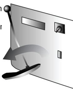
8. At "0" rpm the wheelhead can be turned freely for use as a banding wheel.
